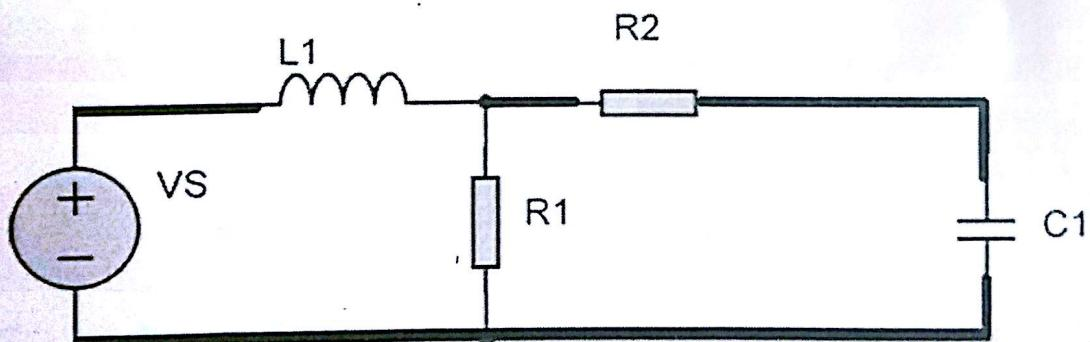
2. Determine the phase variable state space representation in matrix form for the following system and draw the state flow diagram
